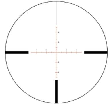
Ultra precision laser etching on the glass reticle ensures that mrad specifications can be kept to the tightest tolerances possible. The fine center crosshair subtensions on the EBR-1 MRAD reticle were carefully chosen to provide the optimum balance between precision aiming and low light visibility.
