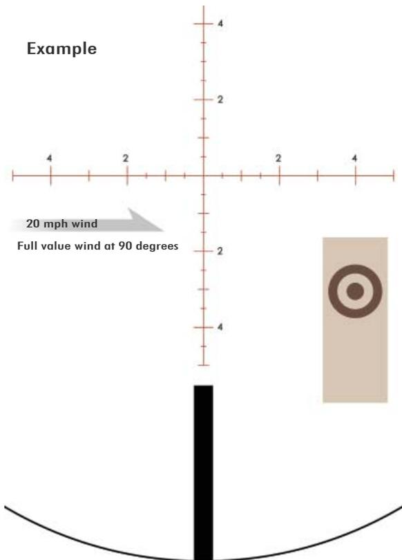
Using 3 mrad drop line at 500 yards, 4 mrad correction for 20 mph wind.
