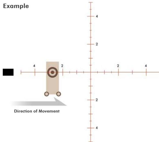
2.74 mrad correction for a target moving at 3 mph at 800 yards. No wind. Total bullet time of flight from trigger pull 1.5 seconds during which target travels 6.6 feet. Elevation already dialed into turret.
